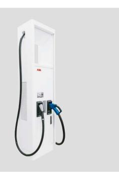
Terra HP is a modular high power charging system with high output current capability, supporting both  $400 V_{DC}$  and  $800 V_{DC}$  vehicles. A single power cabinet system can deliver up to 375 A and 160 kW continuously, and 175 kW peak. With two power cabinets the system delivers up to 500 A and 350 kW.
